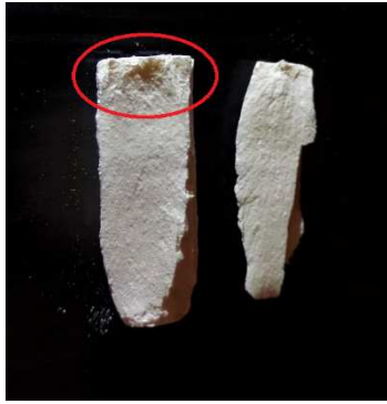
Figure 12. Fracture made in Al35St5 sample consolidated by SCC at 70 °C
